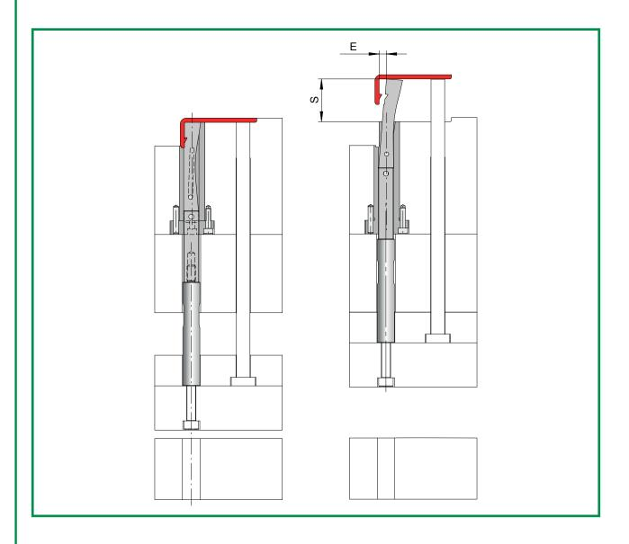
THE LIFTER BODY CAN BE MACHINED ACCORDING TO INJECTED PART GEOMETRY.
