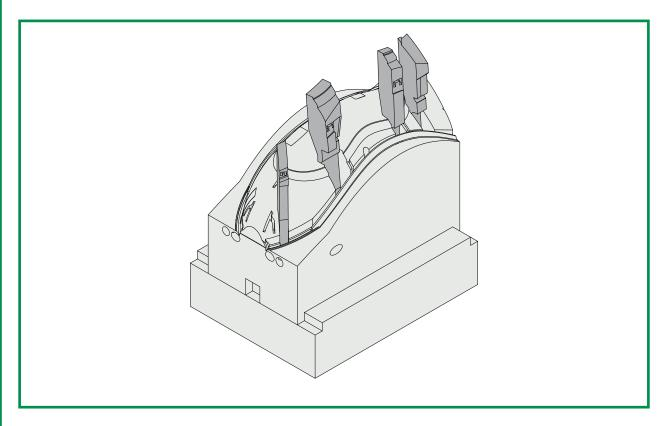
IT IS POSSIBLE TO PRODUCE CUSTOM INSERTS WITH INTEGRATED LIFTERS.
