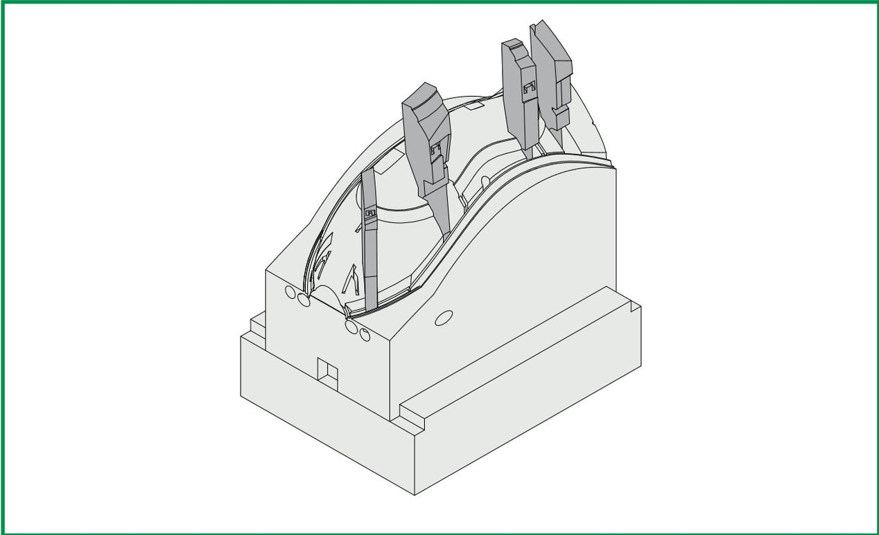
IL EST POSSIBLE DE RÉALISER DES INSERTS SPÉCIAUX AVEC DES CALES ÉJECTRICES INTÉGRÉES.
