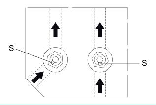
In order to obtain a correct circulation of the coolant, position the fiducial mark S that you can find on the bubble as indicated in the diagram.
