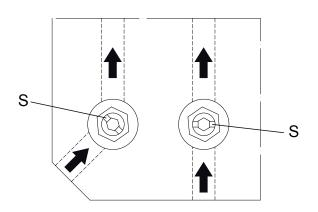
In order to obtain a correct circulation of the coolant, position the fiducial marks S that you can find on the baffle as indicated in the diagram. The fiducial marks correspond to the position of the blade.
