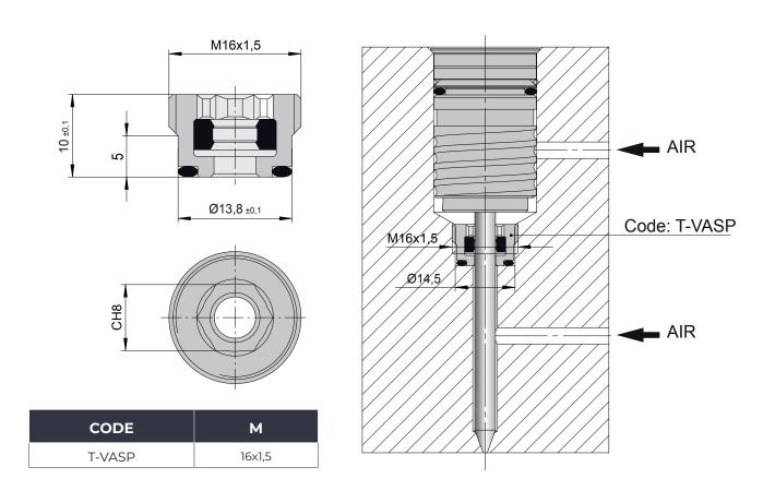
To optimize the operation of the needle valve VASP, it is possible to apply the T-VASP stem seal in order to create a dedicated chamber for retraction that is isolated from the air delivery channel in the cavity. This application can also be useful in case the VASP valve is intended to aspirate air from the cavity to create a vacuum before molding.
